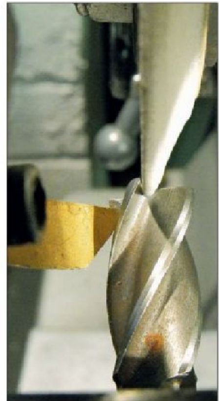
Photo 47. Checking for best wheel fit.
