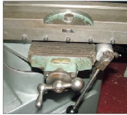
Photo 5. The MK2 slides are protected from grit.
