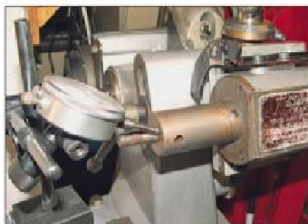
Photo 19. Measuring the run out of the spindle with a DTI.
