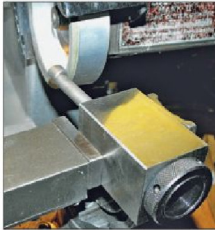
Photo 57. A resin bonded diamond wheel sharpening a carbide tipped boring tool.
