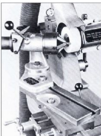
Photo 34. The Clarkson/March drill point and tap lead grinding attachment.
