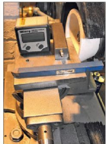
Photo 56. Three way vice set up to grind lathe tools.
