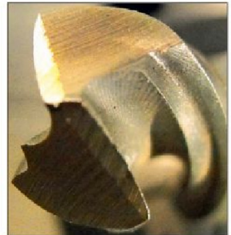
Photo 39. A drill sharpened using the four facet method.
