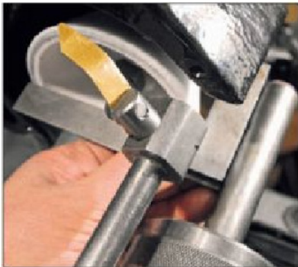
Photo 46. Checking for square.
