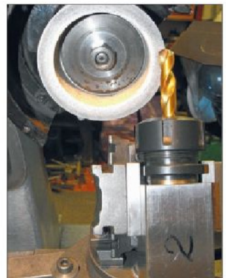
Photo 36. The setup for thinning the web.
