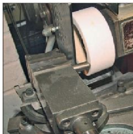
photo 22. I have been using a 0.35 carat diamond in a steel rod held in a three way vice to dress the wheel.
