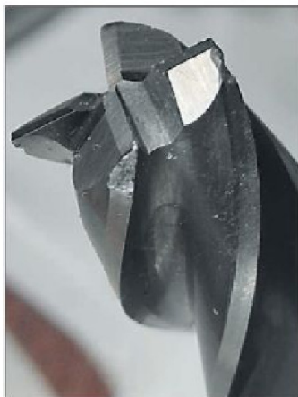
Photo 61. The side of a used carbide end mill.
