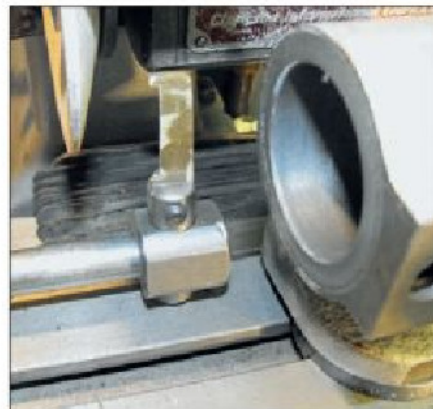
Photo 54. The hook shaped finger for sharpening saws.
