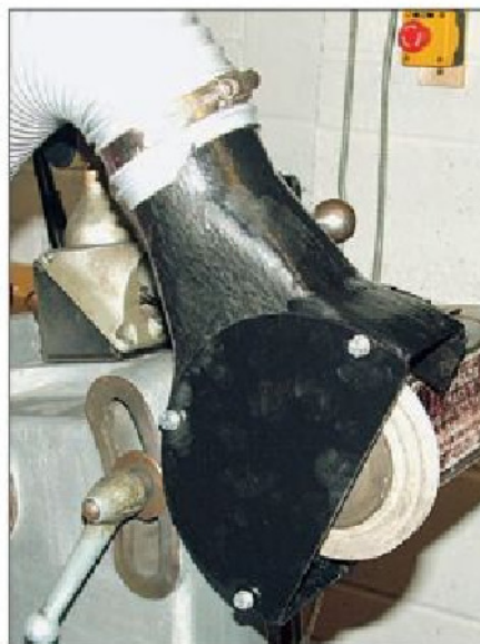
Photo 14. Wheel Guard and Extraction Hose.
