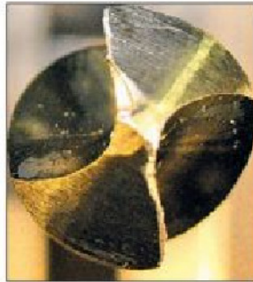
Photo 29. This drill has suffered from severe industrial use.
