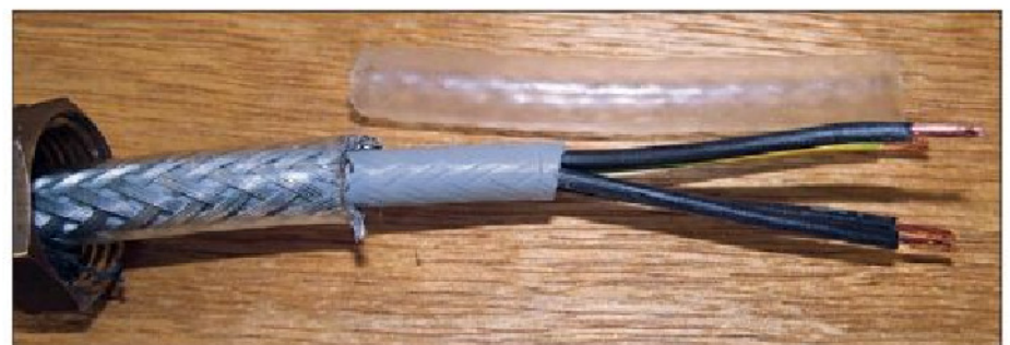
Photo 11. SY Armoured Cable.
