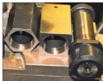
Photo 35. 5C collet holder blocks used for holding cutters.
