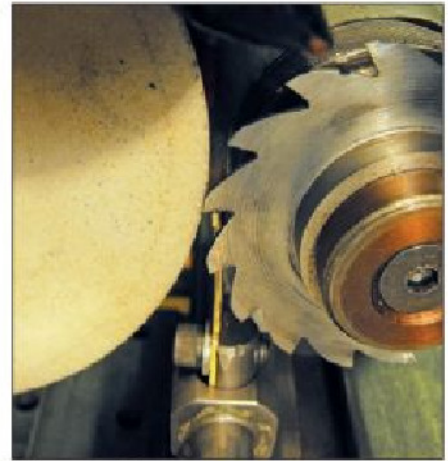
Photo 53. Sharpening a slitting saw.
