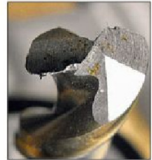
Photo 31. Six facet sharpening.
