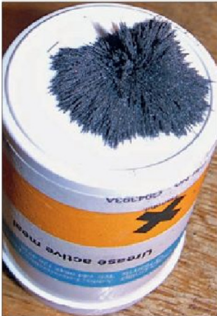
Photo 16. Magnetic Grinding Dust.
