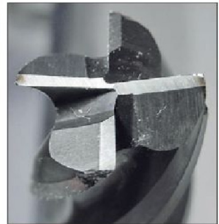
Photo 60. The end of a used carbide end mill.
