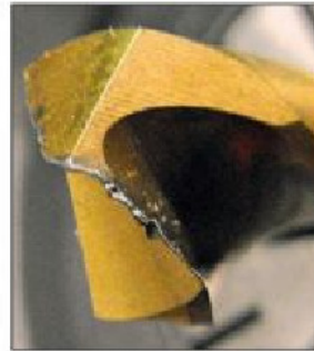
Photo 30. Four facet sharpening.
