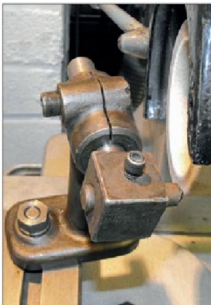
Photo 20. My machine came with a mounted diamond, not a Clarkson one.
